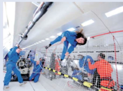
Structural dynamics testing during a parabolic flight, photo credit: German Aerospace Center (DLR)
